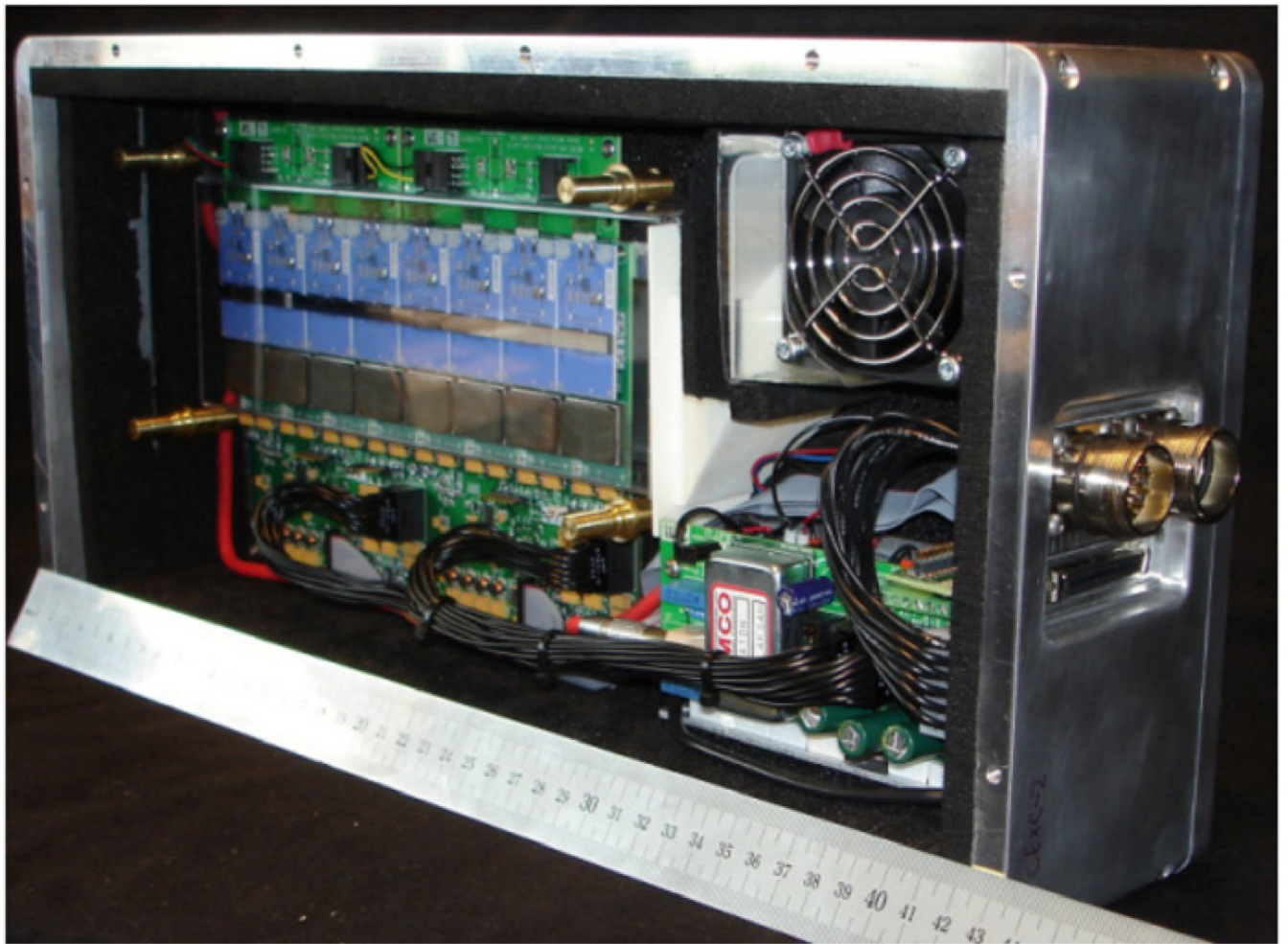
Figure 1. Photograph of the energy-resolved photon-counting x-ray detector.
