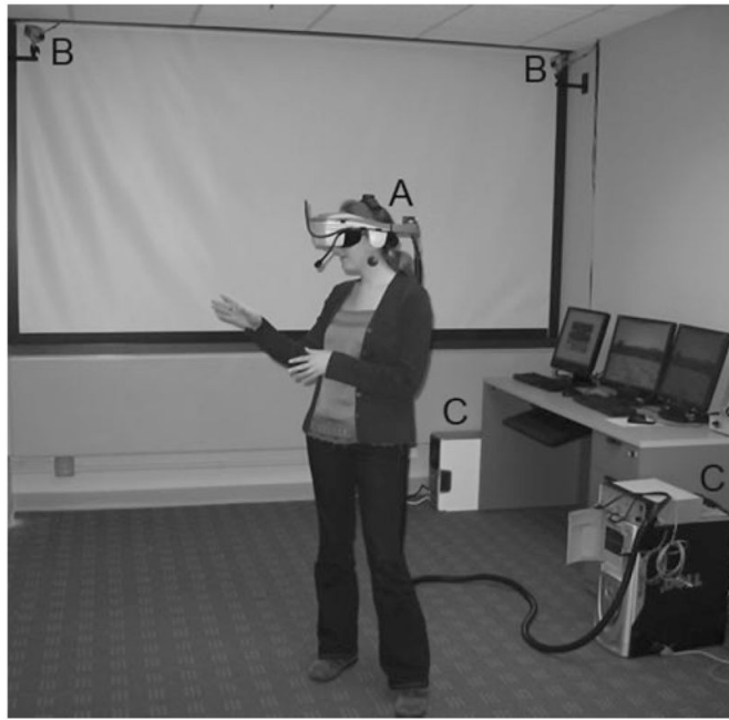
Fig. 1. Illustration of IVE set-up. a Head-mounted display; b tracking cameras; c ) tracking and rendering computers
