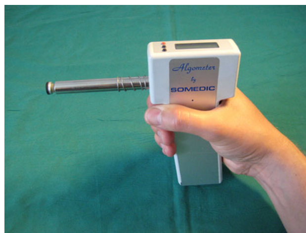
Fig. 1 A hand-held pressure algometer. (Algometer ® , Somedic Sales, Hörby, Sweden). The pressure algometer consists of a 'pistol' handle and a rod with a pressure-sensitive gauge strain at the tip. The applied pressure can be read on a digital display
