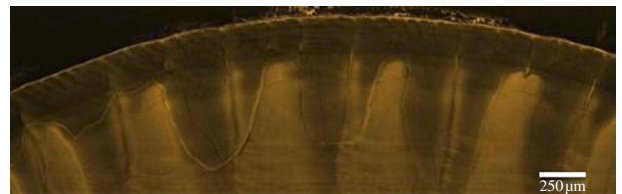
Figure 11. X-ray tomogram showing a perspective view from the bottom of a barnacle base plate showing a crack-arresting fracture pattern. In this case, the fracture occurred through the adhesive and into the mineralized base plate structure. The fracture pattern follows stiffening structures found within the barnacle shell (as shown in the upper left portion of figure 2). (Online version in colour.)
