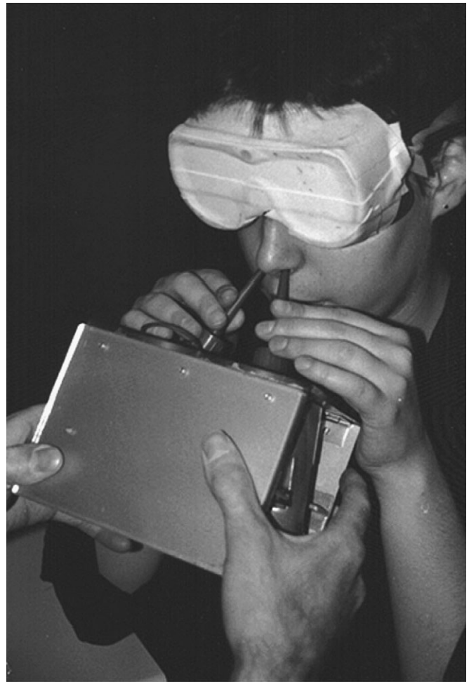
Figure 1 Picture of the stimulus presentation device used in this study (Roscher et al. 1996). The subject is holding onto the spouts of the bottles so that the squeezing of the device would not produce mechanical irritation at the nostrils.
