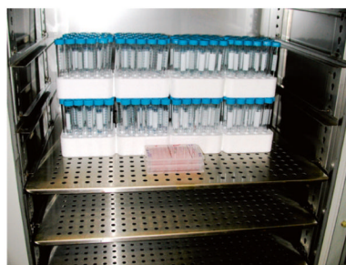
Fig. 8. Comparison of plasticware and incubator space needed for 200 aggregates in 15-ml centrifuge tubes or in 96-well polypropylene plates.
