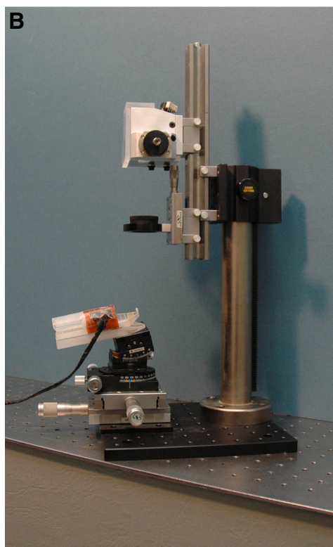
FIGURE 1. (A) Time-domain OCT interferometer and (B) table-top delivery system with mouse-positioning stage.
