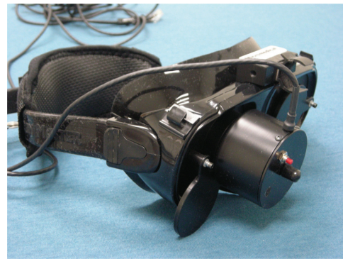
Figure 1 Goggles, with the infrared camera attached to the right eye, manufactured by Micromedical Technologies.
