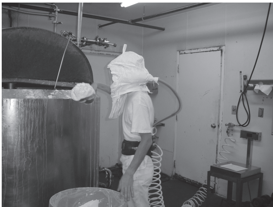
Photo 7: Mixer using supplied-air respirator while manually adding powdered butter flavoring to heated soybean oil in the open mixing tank. Courtesy of the National Institute for Occupational Safety and Health.
