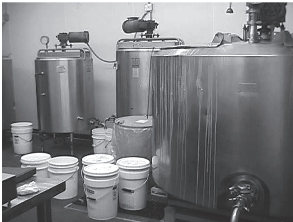
Photo 2: Mixing and flavor-holding tanks before implementation of controls. Note the five-gallon buckets used for open transfer of flavorings, and evidence of spills on outside of the mixing tank. Courtesy of the National Institute for Occupational Safety and Health.
