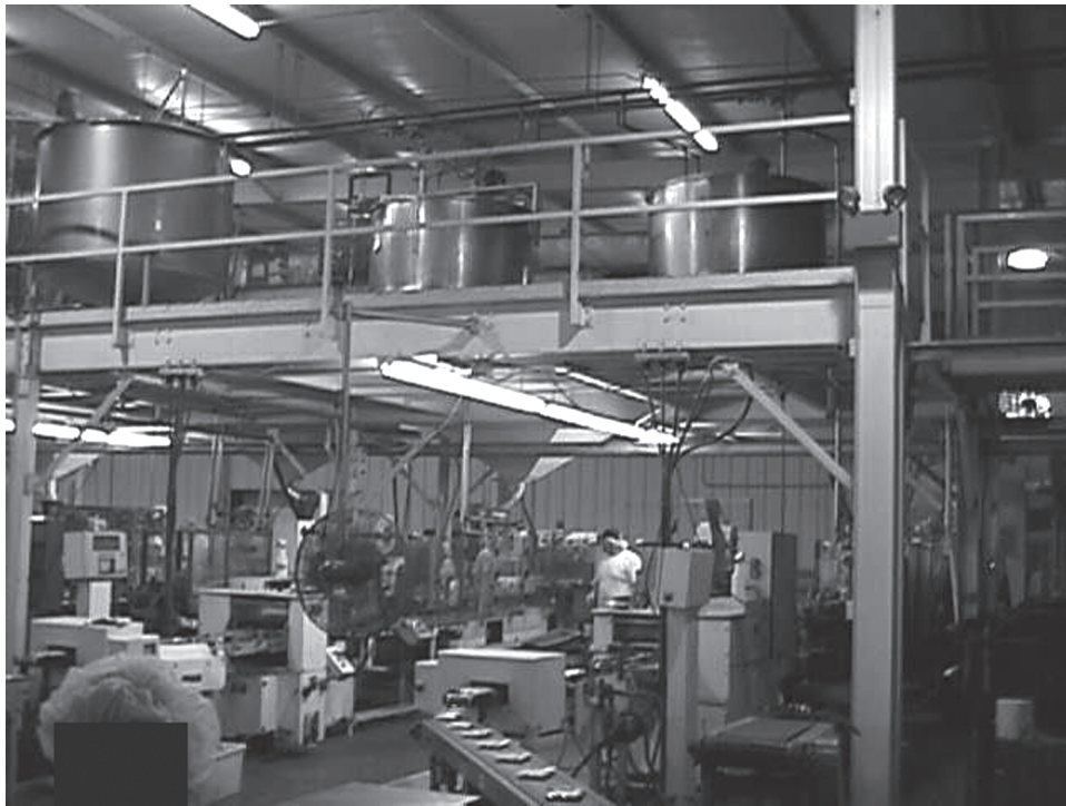
Photo 8: Microwave popcorn packaging line area before implementation of exposure controls. Note heated holding tanks for the oil and flavoring mixture located on a mezzanine above the packaging lines. Courtesy of the National Institute for Occupational Safety and Health.
