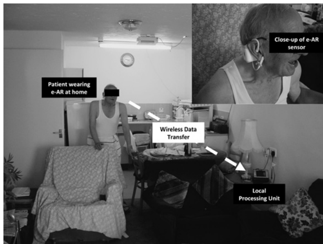
Figure 1 Outline of the architecture of this system, showing the flow of data and a close-up of a sensor being worn by a patient. e-AR, ear-worn activity recognition.
