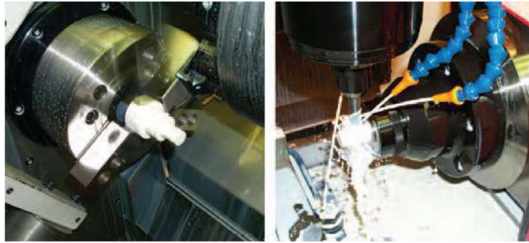
Figure 2. Manufacturing a ceramic part in the CNC lathe and milling machines.
