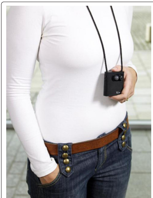
Figure 1 The Microsoft SenseCam digital camera. This wearable device weighs 175 g and passively captures approximately 3,600 first-person point-of-view digital images per typical day.
