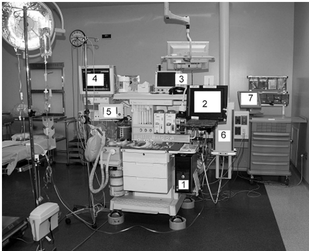
Figure 7. Typical anesthesia workstation including (1) DocuSys computer, (2) DocuSys touch-screen liquid crystal display monitor and keyboard, (3) Bluetooth barcode scanner, (4) physiologic monitor display, (5) anesthesia machine display, (6) movable boom containing outlets for anesthesia gases and network connection, and (7) the Pyxis machine.
