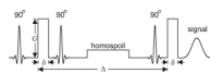
Figure 1. The pulsed-field gradient stimulated-echo NMR pulse sequence. The oscillatory shaped radiofrequency pulses rotate the magnetization by 90 degrees. The rectangular pulsed-field gradients encode the displacement of spins.
