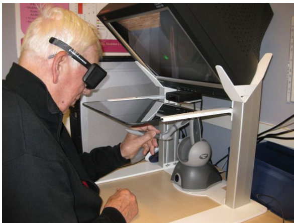
Figure 3 Participant is performing the VR-test. The VR equipment consists of a semi-immersive workbench with haptic device and stereoscopic glasses.
