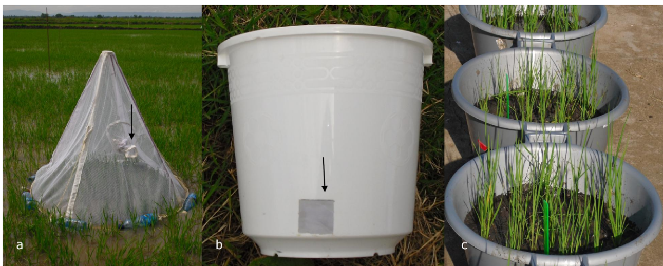
Figure 3. Emergence trap, field bioassay and evaporation measurement. a. Floating emergence trap. Arrow indicates the sleeve used to aspirate the adult mosquitoes and non-target organisms. b. Bucket used for the field bioassay on Aquatain efficacy. Arrow indicates the 25 \text{ cm}^2 holes at the bottom. c. Tubs with 15 rice plants, planted in a 20 cm soil layer. A 4 cm water layer was added to these tubs to measure evaporation. doi:10.1371/journal.pone.0021713.g003
