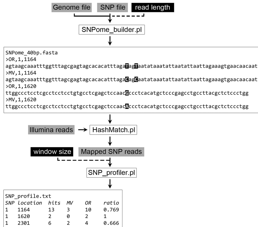
FIG. 1. Pipeline to generate SNPomes and profile SNPs in bulk segregants. The Perl script SNPome_builder creates a SNPome file (shown here for two example SNPs) given a FASTA-formatted genome file, SNP position file, and user-specified read length. SNPs within the SNPome file between OR and MV are highlighted in capital letters. Hashmatch (12) was used to map Illumina high-throughput sequencing reads, the output of which was analyzed by the Perl script SNP_profiler using a 5-kb window size. The output of SNP_profiler indicates the chromosome and position of each SNP, the number of times each version of the SNP was sequenced, and the ratio of the versions in a tab-delimited file.
