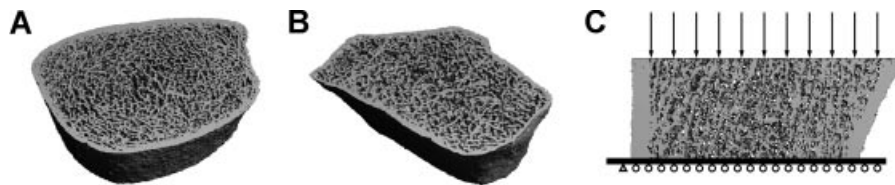
Fig. 1. 3D HR-pQCT images of (A) the distal tibia and (B) the distal radius. (C) Boundary conditions for the FE analyses of both the distal tibia and radius.
