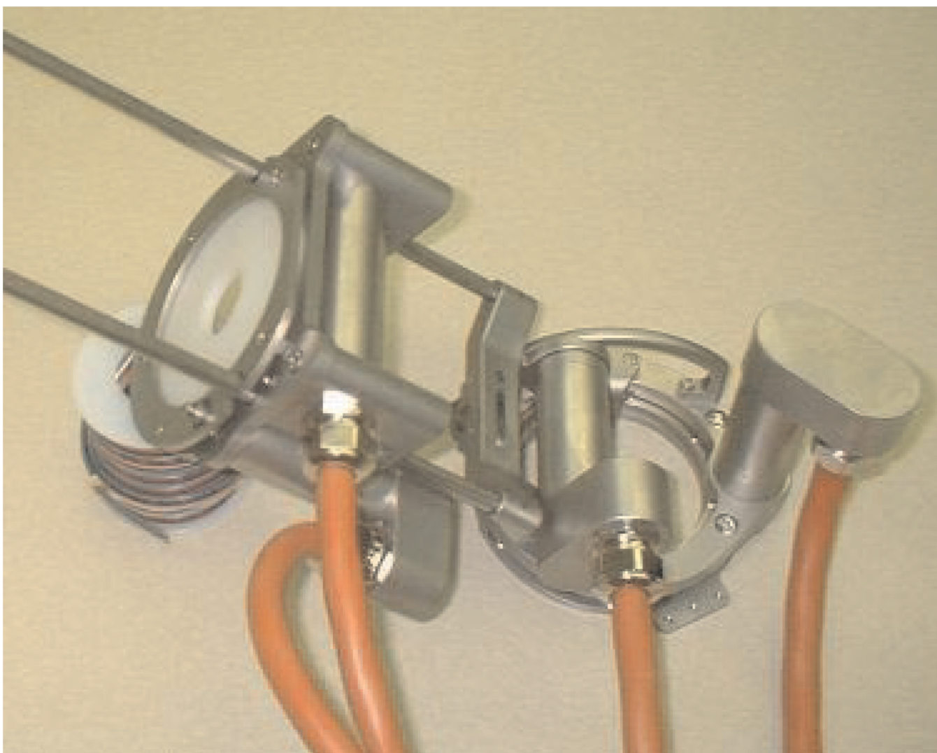
Fig. 7. Instrument manipulator robot prototype.
