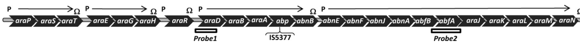
FIG. 1. Genetic map of the 38-kb segment containing the arabinose and arabinan utilization genes. The letter P indicates the proposed promoter site, and Ω indicates the position of the putative rho-independent transcription termination site. DNA probes for the Northern blot analyses are shown as open boxes. Note that the abp gene is interrupted by an ~1.4-kb insertion element, ISS377.
