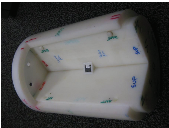
FIG. 3. Inner cylinder of the anthropomorphic phantom, with one quarter removed for dosimeter visualization. The cylinder can hold two dosimeters at a time, each equally spaced 8 mm from the central axis of rotation.
