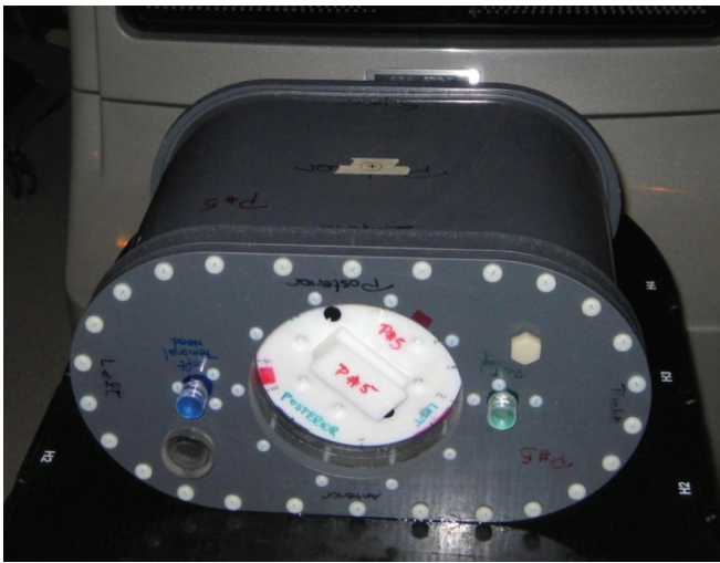
FIG. 2. Radiological Physics Center phantom measuring approximately 38(L) \times 20(W) \times 28(H) cm 3 . The center cylinder rotates within the larger structure to allow irradiation at any angle without moving the setup.
