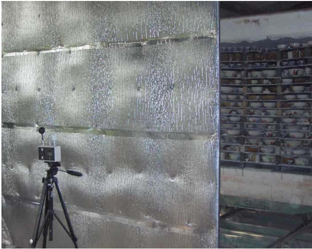
Figure 2: Measurement of thermal conditions behind a heat barrier
