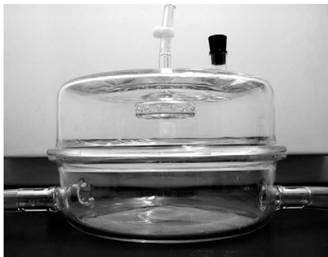
Figure 1. A 3.5-L glass whole body (WB) inhalation chamber for exposing small numbers of rodents to chlorine gas.
