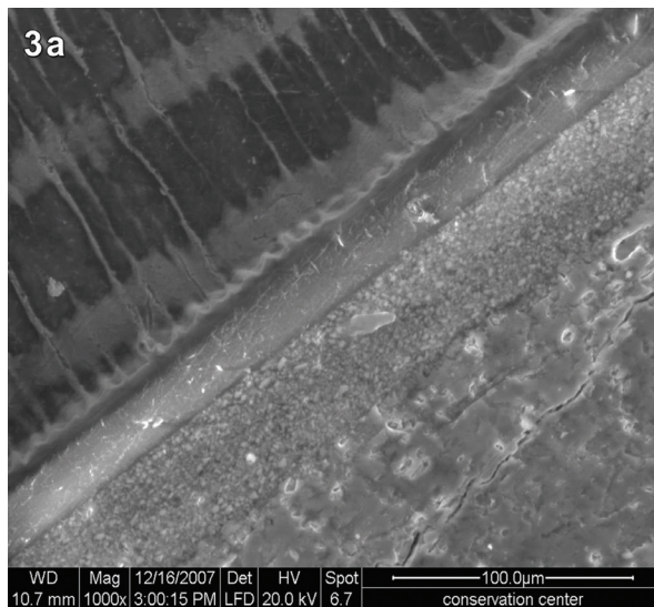
Figure 3. a. SEM micrograph of thermocycled Calibra Resin Cement and b. its corresponding EDAX spectrum curve at one point along the tooth/restoration interface.
