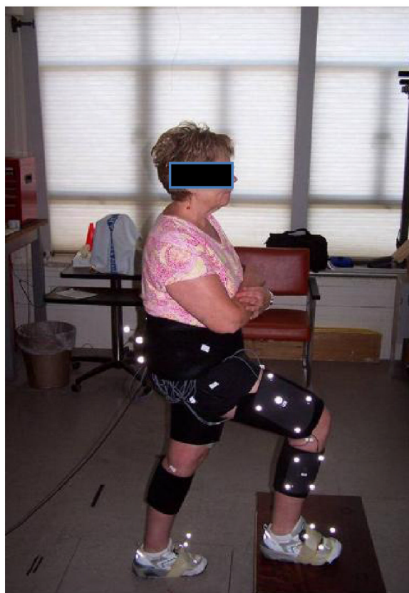
Figure 1. Subject Set up with reflective markers and Instrumented step
