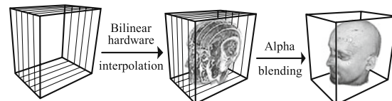
Fig 18. The working pipeline of 2DTM for the 3D dataset ( head ) visualization.
