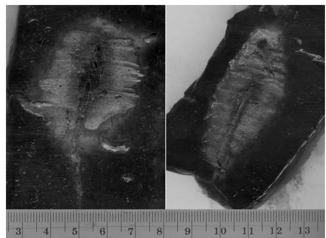
FIG. 11. Ablations created by the optimal dual-slot (left) and monopole (right) antennas in ex vivo bovine liver. Both images presented at equal scale. A total of 50 W at 2.45 GHz was delivered for 10 min in each case. Overall, dual-slot ablations were shorter in length and larger in diameter than monopole ablations.
