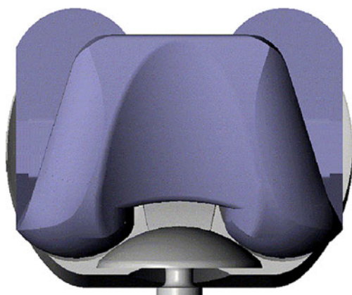
Fig. 1. This is a schematic diagram of the Optetrak total knee replacement system showing the patellofemoral articulation
