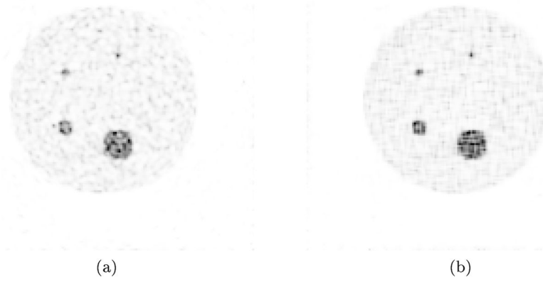
Figure 10. Contrast phantom, reconstructed with 50 iterations of list-mode 3D-OSEM with two subsets, using (a) a shift-invariant Gaussian kernel and (b) a shift-varying model based on the CDRF.
