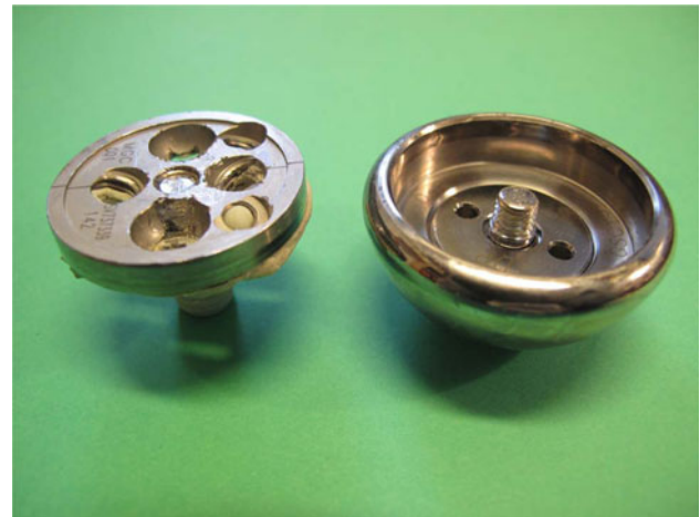
Fig. 2 Glenosphere and metaglene removed from a patient in whom the central screw had broken, creating severe pain.
