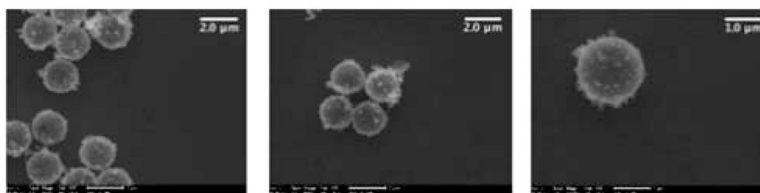
Fig. 3. Three SEM images are of the boron-doped 2 \mu\text{m} shells with increasing magnification (9342 \times , 9354 \times , and 18 708 \times ). Microshells are well formed and virtually no broken shells are observed.
