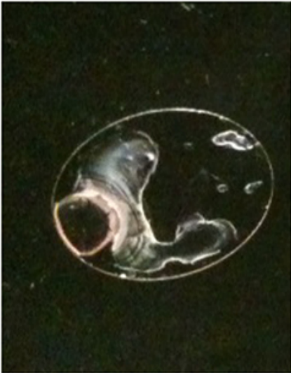
Figure 1A. Improperly washed coverslip. Following addition of APTMS, coverslip was washed for 1-2 minutes before addition of the glutaraldehyde solution. A precipitate forms on the coverslip that has not been washed according to the steps outlined in Procedure.
