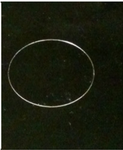
Figure 1B. Properly washed coverslip. Following addition of APTMS, coverslip was washed for three times 10 minutes each before addition of the glutaraldehyde solution. No precipitate forms on the coverslip.
