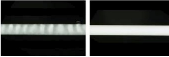
Figure 4. Tendon projection at 105x magnification before and after stretching.
