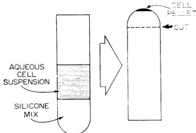
FIG. 1. Relative position of the aqueous cell suspension, the silicone mix, and the location of the pellet and cut. The 10-ml cellulose nitrate tubes for the HS-2 swinging-bucket rotor were obtained from Sorvall. We have recently found that a 12-place fixed 40°-angle rotor (Sorvall SE-12) is also suitable for this purpose. Silicone-washed cells can also be collected in the Sorvall Continuous Flow System by filling the bottom half of each collecting tube with the silicone wash solution.
