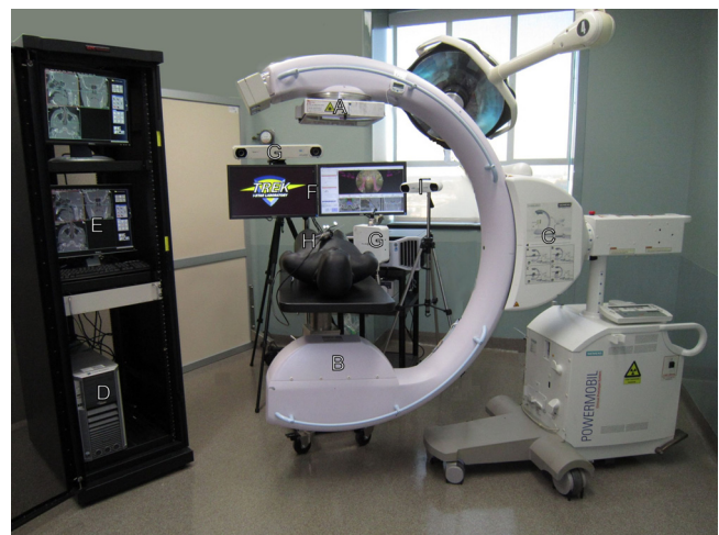
Fig. 1. Prototype C-arm and navigation system for CBCT guidance of surgical interventions. The main components of the C-arm prototype are (a) a flat-panel detector, (b) X-ray tube, and (c) a motorized orbit with computer-controlled x-ray exposure, detector readout, and (continuous) C-arm rotation. CBCT reconstructions are computed using a GPU-based variation of the Feldkamp algorithm, with images available on the acquisition computer (d and e) and integrated with video endoscopy, planning data, and surgical navigation at tableside (f). A variety of endoscopic video and tracking technologies (g–i) are integrated with the system.
