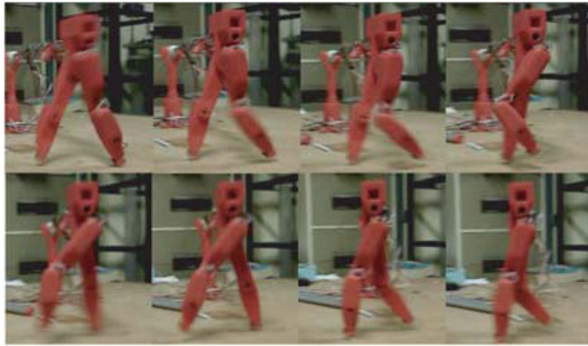
Fig. 13. Redbot [40] bipedal robot walking using the evolved network mimicking human joint angle profiles.
