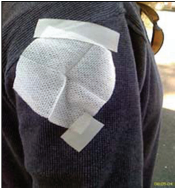
Figure 7. Photograph of a gauze wipe attached to a sampler's arm. Color images available online at www.liebertonline.com/bsp
