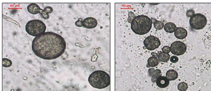
Fig. 1. Photomicrograph of the microsponges prepared by o/o solvent diffusion method
