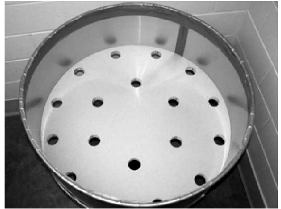
Fig. 3. Odor arena apparatus showing 18 hole positions designed to hold comparison stimulus cups.
