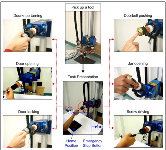
**Figure 1 Current implementation of the tool-changing process and functional task in ADAPT.** Six reach-to-grasp tasks with four different functional task tools were implemented (doorbell: bell pushing; jar: jar opening; doorknob: knob turning, door locking, door opening; screwdriver: screw driving).
