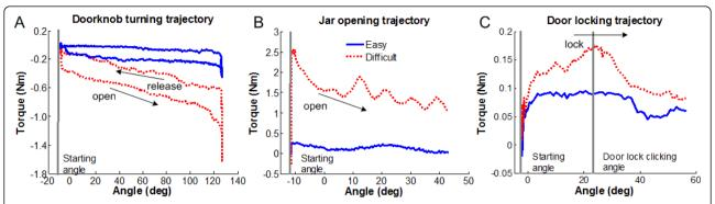
**Figure 3 Sample trajectories of functional tasks.** Torque versus position trajectories are plotted for three functional tasks in the training session. The blue solid line shows the trajectory of each task at lowest difficulty, which is selected in the first trial of the training session. The red dot line is the trajectory of each task at high difficulty, which is selected near the end of the training session.
