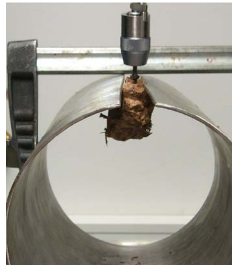
Fig. 2 Steel fixation device. The screw head was attached by using an AO Universal Instrument
