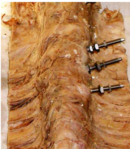
Fig. 1 Human cadaveric spine with implanted anterior vertebral body screws T9-11. Upper screw: non-augmented vertebra; middle screw: screw implantation in soft cement; lower screw: screw implantation in cured cement
