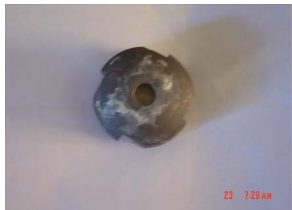
Fig. 8 Cup showing complete delamination
