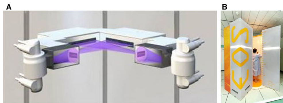
Fig. 4 a Principle of the EOS system with the two orthogonal tubes, their fan-shaped collimated X-ray beams and the two collimated detectors. b EOS system gantry with the patient inside
