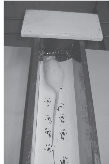
FIGURE 2: Walking track apparatus. Rat in an 8.2 \times 42 cm walking track apparatus lined with white office paper. After the hind limbs of the rat are dipped in Chinese ink, the rat walks towards the darkened end of the corridor.
