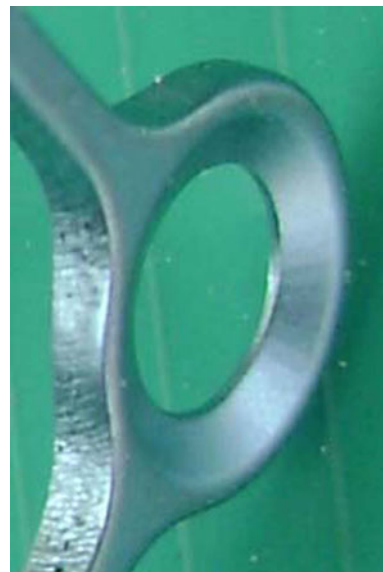
Fig. 3 Bevel in the plate to engage the thread in the screw head
