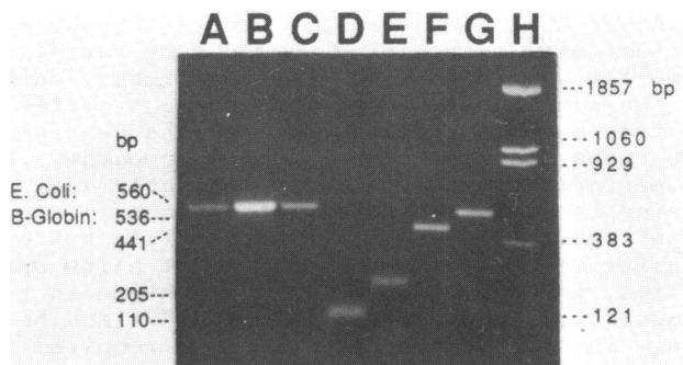
Fig. 4 Ethidium bromide stained amplification products. Lane A shows the product of amplification in microfuge tubes manually transferred between water baths for comparison to the hot air amplifier in lanes B-G. Lanes A-C) 560 bp fragment of E. coli DNA defined by primers TGAATCTGTACTCTGATGTAAC and CACTAATAGCAAGAGGGTACTCAG covering a portion of the regulatory region for pyelonephritis-associated pili (6). An asymmetric amplification (50 pmol of one primer and 0.5 pmol of the other) is shown in lane C. Lanes D-G) Amplification products of 4 different combinations of the human beta-globin gene primers PC03, PC04 (7), KM29, and RS42 (8). Lane H) Bst N I digest of PBR322 DNA size markers (0.5 ug).
