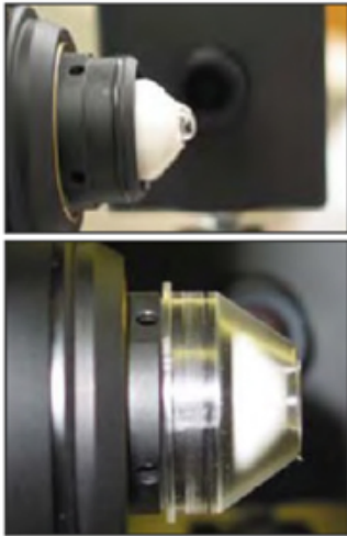
Figure 1. Preparation of the objective lens tip (top) applying viscotear gel (bottom) Applying the TomoCap.
