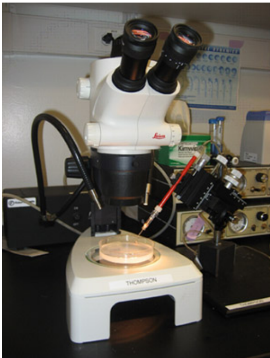
Figure 1. Electroporation station. Electrodes were made using sharpened 75 \mu m Tungsten wires and connected by leads to a Protect CUY-21 Edit Square Wave Electroporator. These electrodes were taped to micromanipulators.
