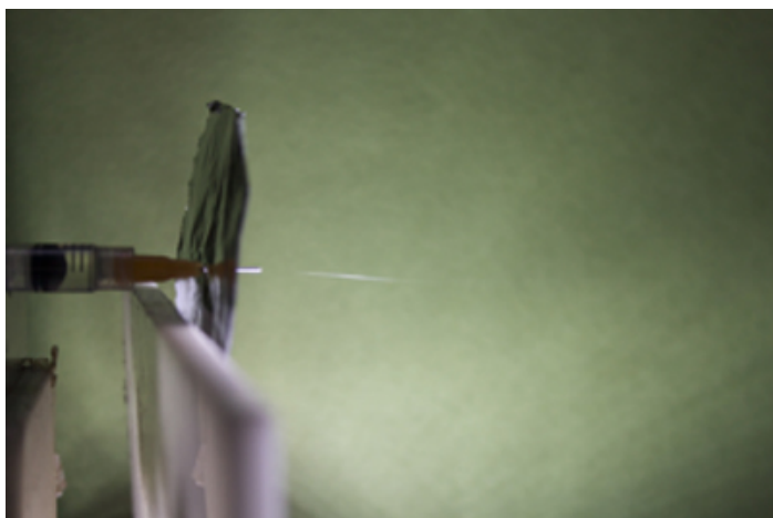
Figure 2. The streaming jet is visible exiting the syringe tip; the whipping jet is too small to be seen.
