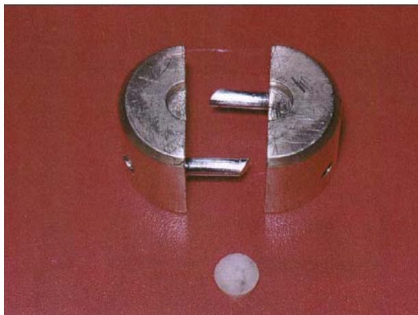
**Fig 1.** The metallic mold used for preparing the specimens.
